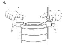
down simultaneously to ensure the clamping plate is square. Continue until the handwheels are tight against the internal stop. Hand tightness must be exerted so that the assembly does not loosen during vibration.
