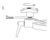
Ensure that the clamping handwheels at the top are loose and the locking assemblies are fully pushed down. There should be a 5mm gap between the large plain washer and the face of the handwheel.
