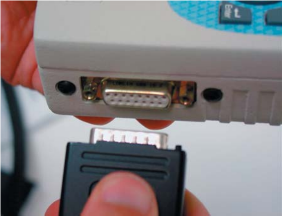
Carefully mate the connector on the SLC or STS sensor to the connector on the side of the DFS-R-ND gauge.
