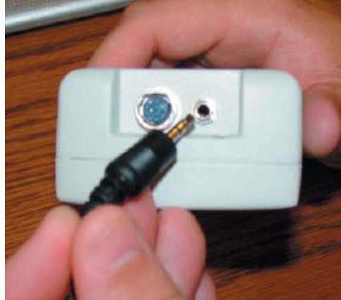
Connect Stereo Connector to top of gauge.
