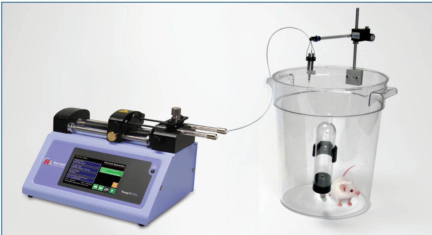
Harvard Apparatus offers a complete Glucose Clamp Infusion System for rats or mice including syringe pumps, swivels, tethers and catheters. Multiple syringe pumps push glucose, insulin and a drug, tracer glucose or other fluids into a 3 or 4-way connector which combines and reaches the animal via one channel
