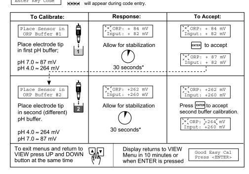
\* For best results, gently stir the submerged electrode for approximately 5 seconds during the stabilization period. Large temperature differences from process fluids to buffers may require longer stabilization time.
