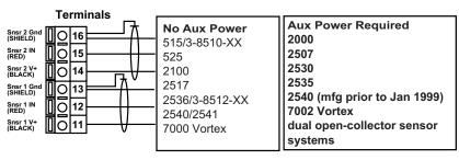
Maximum cable length is 200 ft. for 515/8510-XX, 525, 2517 and any sinusoidal flow signal.
