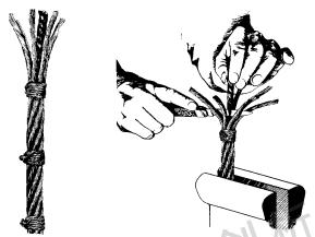
FIG. 1 Wire Rope for Socketing, (a) and (b)
