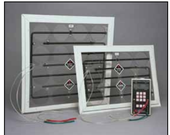
The TrueFlow® Air Handler Flow Meter, shown with DG-700, is used to measure the total amount of air moving through an air handler.
