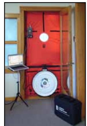
DG-700 Pressure and Flow Gauge with Cruise feature
