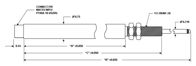
Dimensions are in inches (Refer to mechanical specifications for dimensions "A", "B" and "C")
