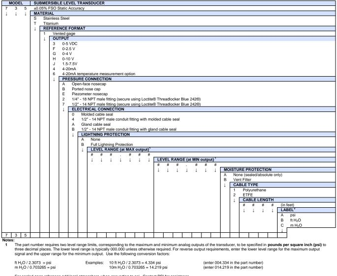
For sealed gage reference add local atmosphere when converting to psi. Contact PSI for assistance. Example: 10 ft H<sub>2</sub>O / 2.3073 +14.7 = 19.034 psi
