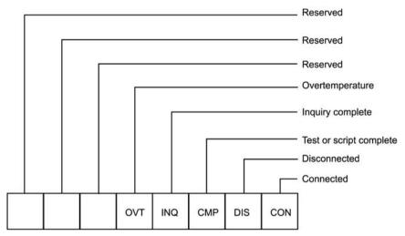
The INS register displays the present status of the instrument and can be used to provide SRQs for test or script completion and the connection status of the instrument by setting the corresponding bits in the INE register
