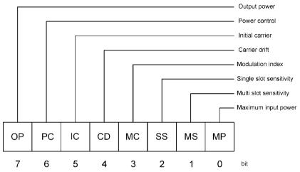
This EUT register is cleared on the start of a test or script. When a test completes, if it has failed the test limit parameters enabled to give a fail result the corresponding bit in this register will be set. These events can be programmed to provide an SRQ by setting the corresponding bit(s) in the Equipment Under Test Fail Enable Register (ETE).
