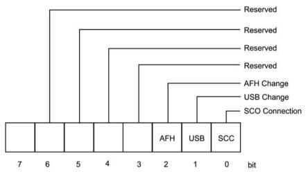
The CHG register indicates when a change of state has occurred in the instrument, and can be used to provide SRQs by setting the corresponding bits in the CHE register.
