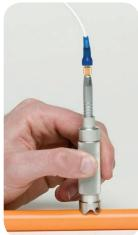
The Sonopen<sup>®</sup> transducer has a replaceable delay line that is tapered to a small contact area. This transducer makes reliable thickness measurements in applications such as turbine blades, threads on plastic bottle necks and tight radii on plastic containers. High-temperature Sonopen delay lines are also available.
