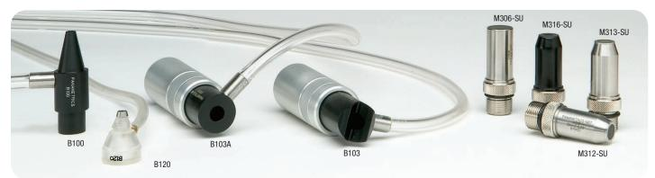
Panametrics Microscan immersion transducers are designed to transmit and receive ultrasound in water. Thickness measurements by immersion technique are often preferred when the test piece has a complex geometry or in online applications. Typical offline applications include wall thickness measurements on small diameter plastic or metal tubing, scanned or rotary measurements and thickness measurements on sharply curved parts. Transducer focusing may be necessary depending on the application.
