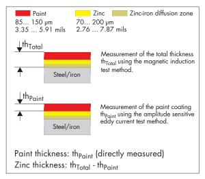
Determining the single coating thicknesses at the duplex measurement using the amplitude sensitive eddy current and the magnetic induction test methods
