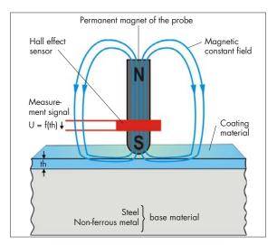
Schematic diagram of the magnetic test method. The indentation depth of the magnetic field depends on the permeability of the base material.
