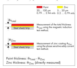
Determining the single coating thicknesses at the duplex measurement using the phase sensitive eddy current and the magnetic induction test methods
