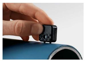
Measurement of the corrosion protection coating in plastics on steel pipes with the probe FKB10
