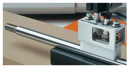
Automated measurement of the chrome coating on piston rods with the probe  $\ensuremath{\mathsf{V2FGA06H}}$
