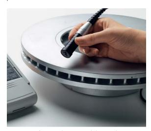
Measurement of zinc powder coating with the two-pole probe  $\it V7FKB4$
