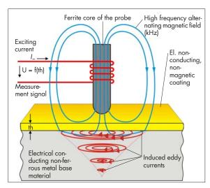
Schematic diagram of the amplitude sensitive eddy current test method. The indentation depth depends on the used frequency and the electrical conductivity of the base material.
