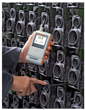
Measuring with the internal probe FAI3.3-150
