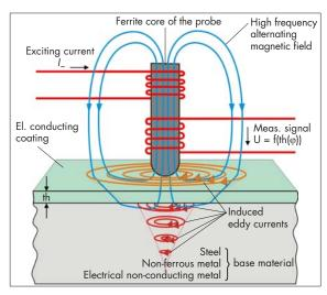
Schematic diagram of the phase sensitive eddy current method. The indentation depth of the magnetic field depends on the used frequency and the electrical conductivity of the materials.
