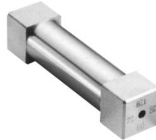
Fig. 9 Film Applicator BAKER 286
