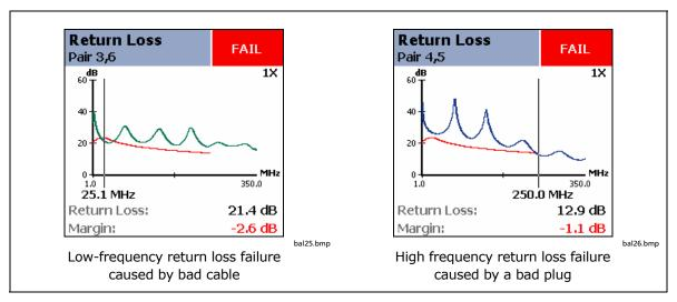
Figure 2. Return Loss Failures at Low and High Frequencies
