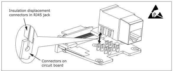
Figure 3. Replacing the RJ45 Jack
