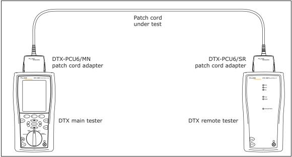
**Figure 1. Patch Cord Test Connections**
