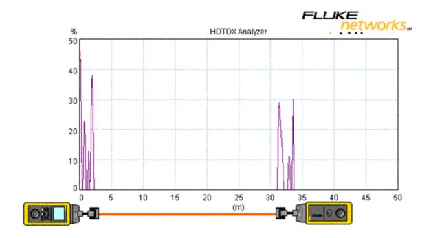
This shows where the crosstalk is happening in the link (High Definition Time Domain Xtalk). The DSP will then convert this Time Domain Trace in meters to a Frequency Domain Plot in MHz as required by the standards for certification shown below:
