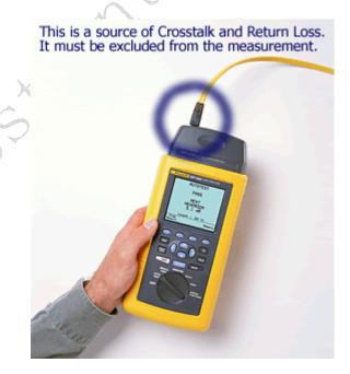
The DSP series from Fluke Networks does this using Digital Signal Processing. The measurement is first made in the Time Domain (feet and meters). An example is shown below:
