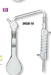
E Kuderna-Danish Concentrators boil away samples to allow testing for pesticides or other pollutants prior to instrumental analysis. Include three-ball Snyder column with venting dimples and graduated collection tube. Available with or without springs mounted on collection tube.
