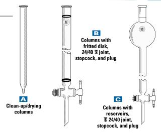
■ LabGlass Columns with Reservoirs are perfect for flash chromatography applications. Includes a PTFE plug to control flow rate.
