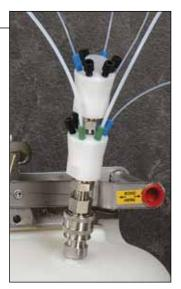
Manifold 86394-27 attached to 86394-31 "stacker"
