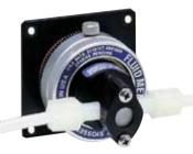
RHO.CTC / FMI 006 Ceramic Tefzel<sup>®</sup> Ceramic Rulon AR PTFE 100°C 6.9 bar 2 fixed tube fittings for PTFE tubing 6 mm o.d.
