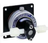
RH1.CKC / FMI 007 Ceramic Kynar (Fluorocarbon {PVDF}) Ceramic Rulon AR PTFE 100°C 6.9 bar 2 fixed tube fittings for PTFE tubing 6 mm o.d.
