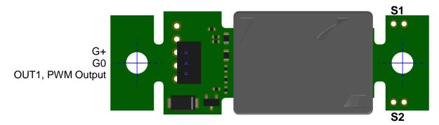
Figure 3: Pin assignment SenseAir® S8-PWM
