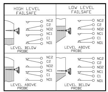
Figure 2. High/Low Level Failsafe
