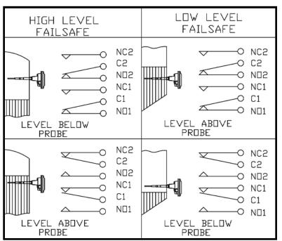
Figure 2. High/Low Level Failsafe
