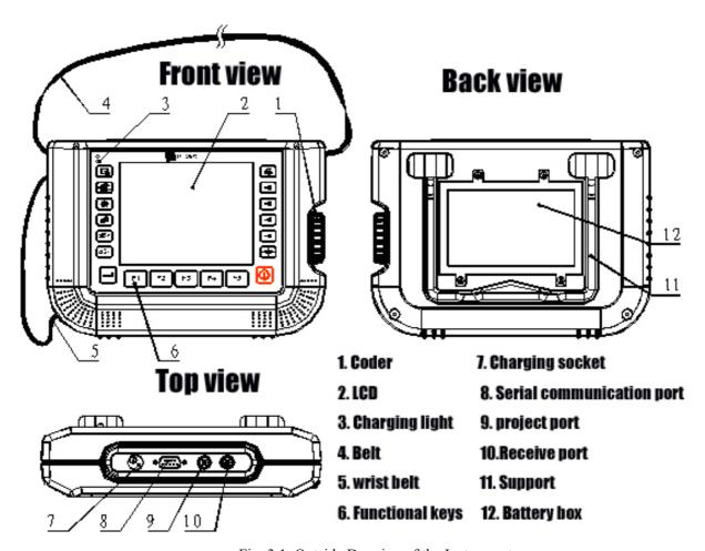
Fig. 3.1 Outside Drawing of the Instrument
