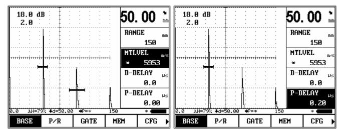
Increase MTLVEL, till the displayed pitch interval between the primary and secondary echo is 50mm, now we get the exact sound velocity of the material, i.e. 5953m/s;
