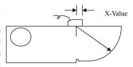
locate the probe on test block and move it as the right figure to make sure you have got the highest echo on R100mm reflector, measure the distance, which is the X-Value of probe, between the front face of probe and cycle center of R100m arc. The point corresponding to the cycle center of R100mm arc is just the incidence point of probe.
