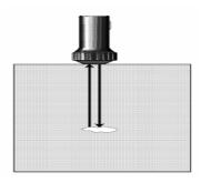
Fig. 1.1Basic working principle for ultrasonic detection
