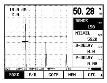
MTLVEL is unknown, set the approximate MTLVEL as 5920m/s, set the Gate Logic as double gate mode, meanwhile set the P delay as 0;
