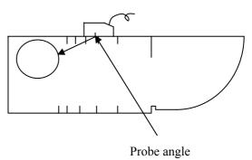
of 74~80 degrees. And on the upside of CSK- I A test block probe of K2.0, K2.5, K3.0 can be calibrated, the downside is suitable for probe of K1.0, K1.5). locate the probe as the right figure shows, move the probe back and forth to make sure you have got the highest echo, and now the scale corresponding with incidence point is the probe angle or K-Value.
