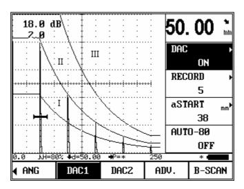
The screen is divided into three areas, I, II and III. The three curves will be drawn on the screen during the detecting, users can determine the flaw character by the height of the echoes.
