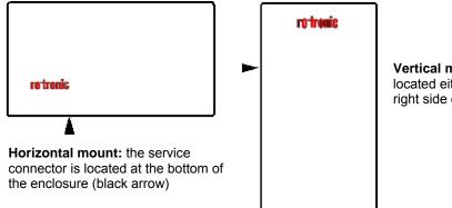
**Vertical mount:** the service connector is located either on the left side or on the right side of the enclosure.
