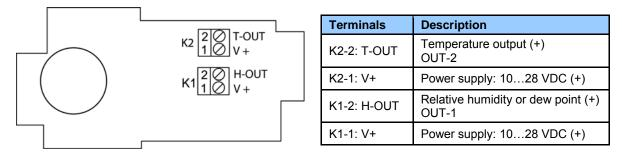
**Note:** connect the + of the power supply to only one of the V+ terminals. The two terminals marked V+ are internally connected.
