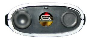
**WARNING**: the service connector is a UART interface with a mini-USB connector type. Do not connect the service connector directly to the USB port of a PC or hub.
