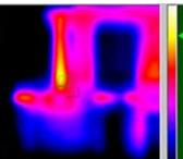
The TMTI 300 is used to show a difference in temperature between two running bearings. This temperature difference could indicate a potential bearing problem that could lead to a failure and downtime
