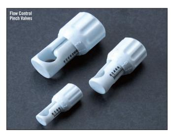
The Flow Control Pinch Valves work with tubing from 5/32 inch OD to 3/8 inch OD. The micrometer dial offers easy resetting of clamping distance. These valves are made of Delrin® and Acetal.
