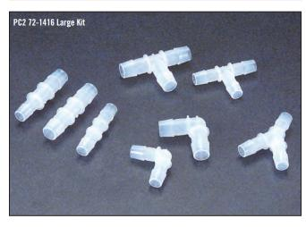
These barbed connector kits come in three different sizes. Small and medium kits have 10 pieces of each component and large kits have 5pieces of each component. Connectors join tubing of similar sizes while reducing adapters join tubing of different sizes. These kits are available in black nylon, polypropylene, and Kynar®, a chemically resistant autoclavable plastic. Each kit is supplied in a convenient box. All kit components are also sold separately.
