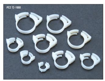
The clamps in the Tubing Clamp Kit feature a simple-to-use ratcheting design which provides positive and secure clamping of tubing to barbed and non-barbed connectors. Thirteen different clamps provide clamping for tubing sizes from 1/16 inch OD to 1.5 inches OD. This kit is supplied in a convenient box containing 5 of each clamp size.
