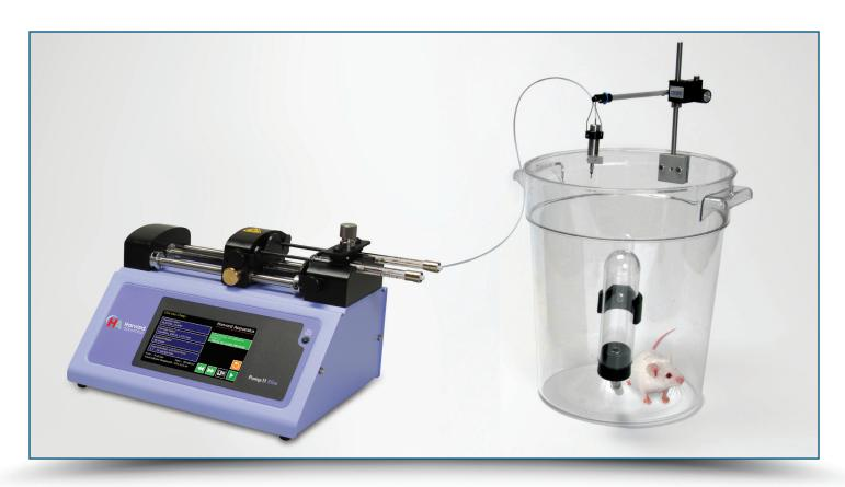
arvard Apparatus offers a complete Glucose Clamp Infusion System for rats or mice including syringe pumps, swivels, tethers and catheters. Multiple syringe pumps push glucose, insulin and a drug, tracer glucose or other fluids into a 3 or 4-way connector which combines and reaches the animal via one channel
