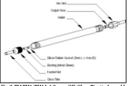
Fig. 3. PLI-PH1/PH1A 1.0 mm OD Glass Pipette Assembly
