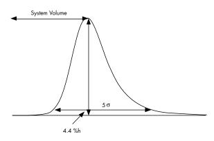
In a typical HPLC system, the Band-spreading Volume should be no greater than 100  $\mu$ L ± 30  $\mu$ L (or Variance of 400  $\mu$ L<sup>2</sup> ± 36  $\mu$ L<sup>i</sup>).In a microbore (2.1 mm i.d.) system, the Band-spreading Volume should be no greater than 20 to 40  $\mu$ L (or Variance no greater than 16  $\mu$ L<sup>2</sup> to 64  $\mu$ L<sup>2</sup>).
