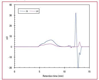
The analyzed result of P(S-B) copolymer was  $5.5 \times 10^5 \text{g/mol}$ , with a polydispersity index of 3.17. The calculated area ratio of UV/RI was 0.44. The calibration curve can be generated from two points, from two copolymers with known composition percentages. Also, a one-point calibration curve going through the origin is acceptable. *Figure 2* shows the one-point calibration curve generated from the P(S-B) copolymer.
