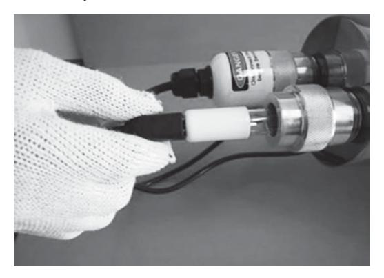
Remove 4-pin Electrical Socket from Lamp Pins. 5.
