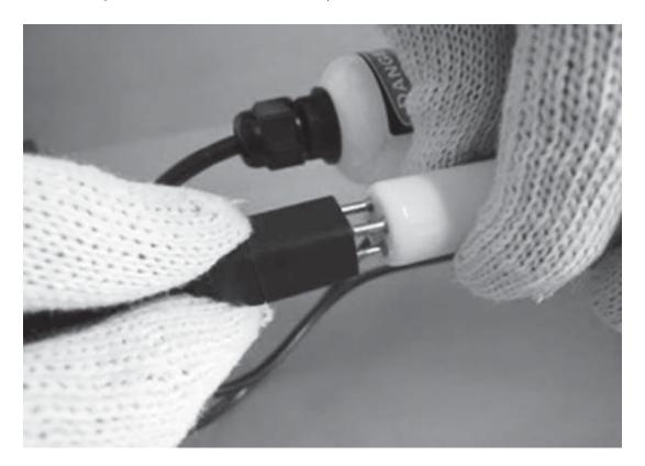
Install the Cover Cap (PC) and Tighten Electrical Cable Gland Connector & Setscrew.
