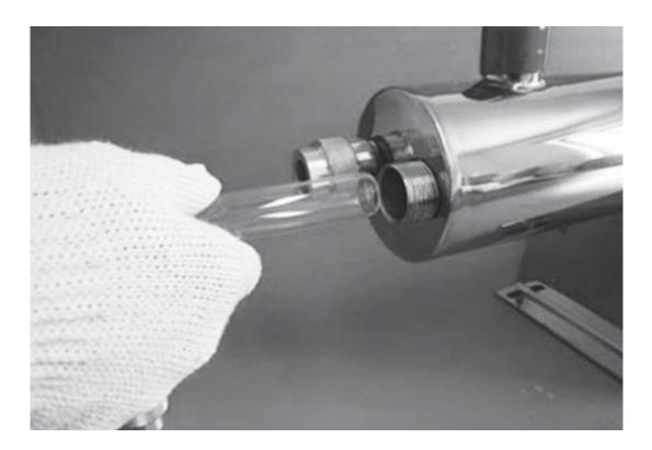
Install O-ring and Washer on both ends of Quartz Sleeve and Be sure O-rings are placed 4. on quartz sleeve before Washer.
