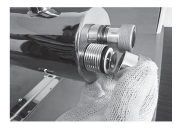
Slide UV Lamp into Quartz Sleeve carefully. Be sure to slide into quartz sleeve without 6. angling.
