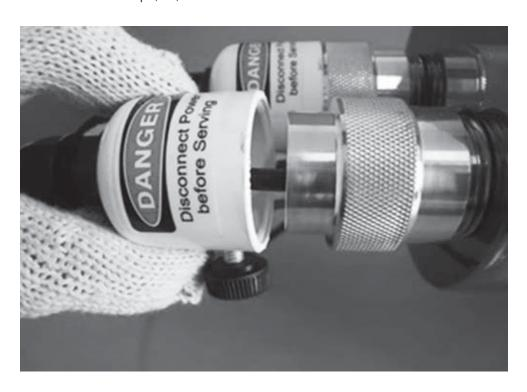
Withdraw wire with lamp carefully until approximately 2 inches of the lamp is exposed. Lamp base can be very hot - be careful not to drop the lamp into the quartz as both are easily broken.
