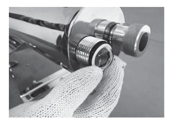
Reinstall Nuts on both sides of reactor chamber. Tighten nuts firmly by hand only. DO NOT USE HAND TOOLS. Tightening with hand tools is likely to cause quartz sleeve to break.
