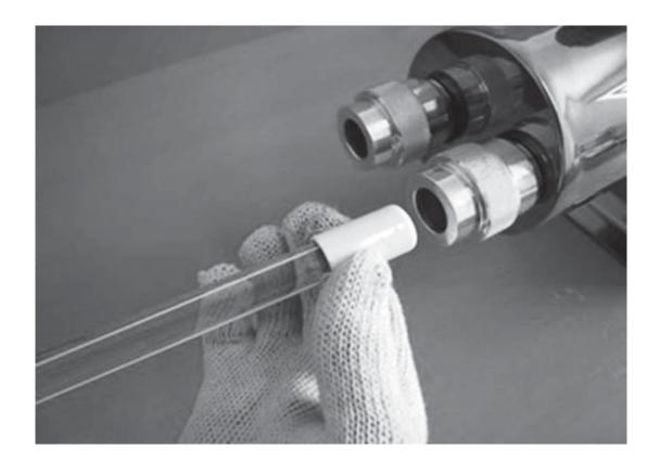
Connect 4-pin Electrical Socket with Lamp. 7.
