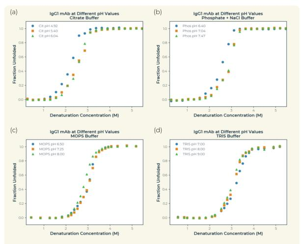
**Figure 2** – Fraction unfolded values against denaturant concentration for each pH value measured. The plots are grouped by buffer, with (a) for citrate, (b) for phosphate, (c) for MOPS and (d) for TRIS.
