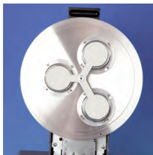
Triple sputtering head with automatic shutter closed
