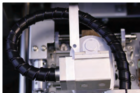
Ultra Coolstage. Range: -50°C to +50°C at 300Pa
