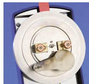
Metal evaporation insert (set up for downwards evaporation)
