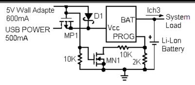
Fig.5:Combining Wall Adapter and USB Power
