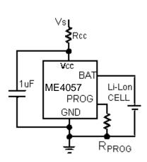
Fig.3:A circuit to maximum the thermal regulation charge current
