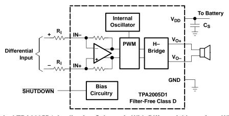
Figure 26. Typical TPA2005D1 Application Schematic With Differential Input for a Wireless Phone
