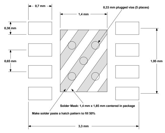
Figure 33. TPA2005D1 8-Pin QFN (DRB) Board Layout (Top View)
