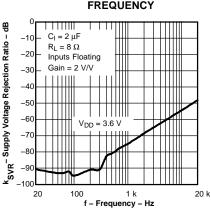
SUPPLY VOLTAGE REJECTION RATIO vs
