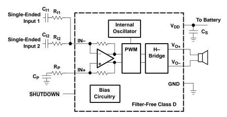
Figure 31. Application Schematic With TPA2005D1 Summing Two Single-Ended Inputs
