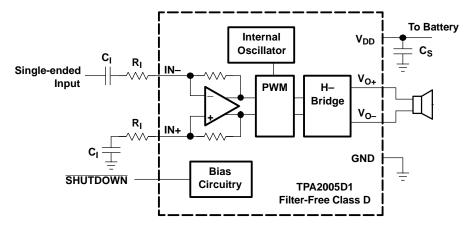
Figure 28. TPA2005D1 Application Schematic With Single-Ended Input
