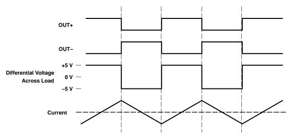
Figure 34. Traditional Class-D Modulation Scheme's Output Voltage and Current Waveforms Into an Inductive Load With no Input
