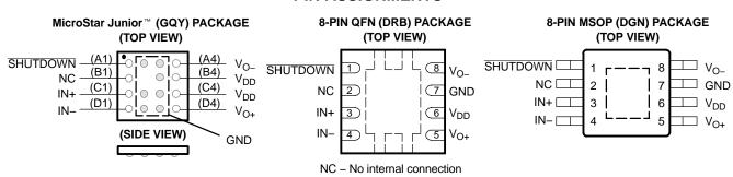
NOTES A. The shaded terminals are used for electrical and thermal connections to the ground plane. All the shaded terminals need to be electrical connected to ground. No connect (NC) terminals still need a pad and trace.
