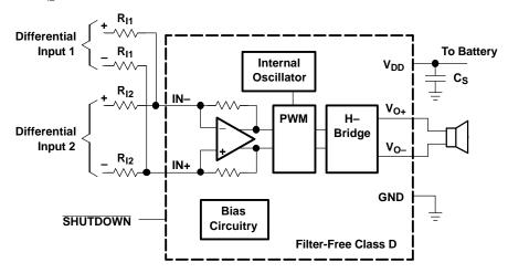
Figure 29. Application Schematic With TPA2005D1 Summing Two Differential Inputs
