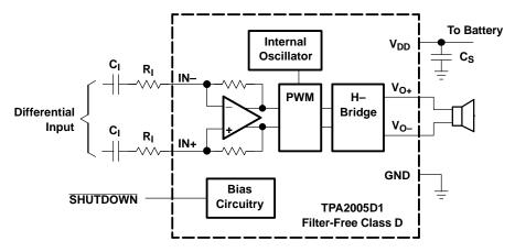
Figure 27. TPA2005D1 Application Schematic With Differential Input and Input Capacitors
