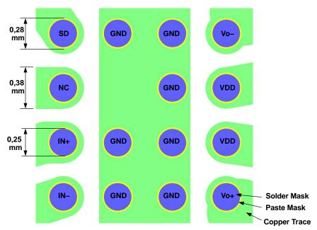
Figure 32. TPA2005D1 MicroStar Junior BGA Board Layout (Top View)
