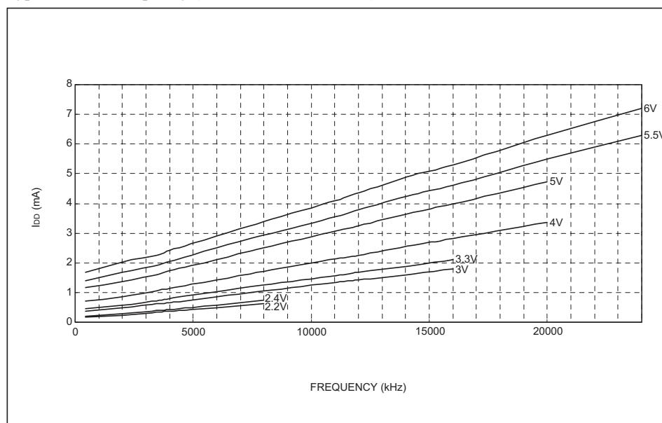
**Typical I<sub>DD</sub> vs. Frequency (External Clock, Ta=+25°C)**
