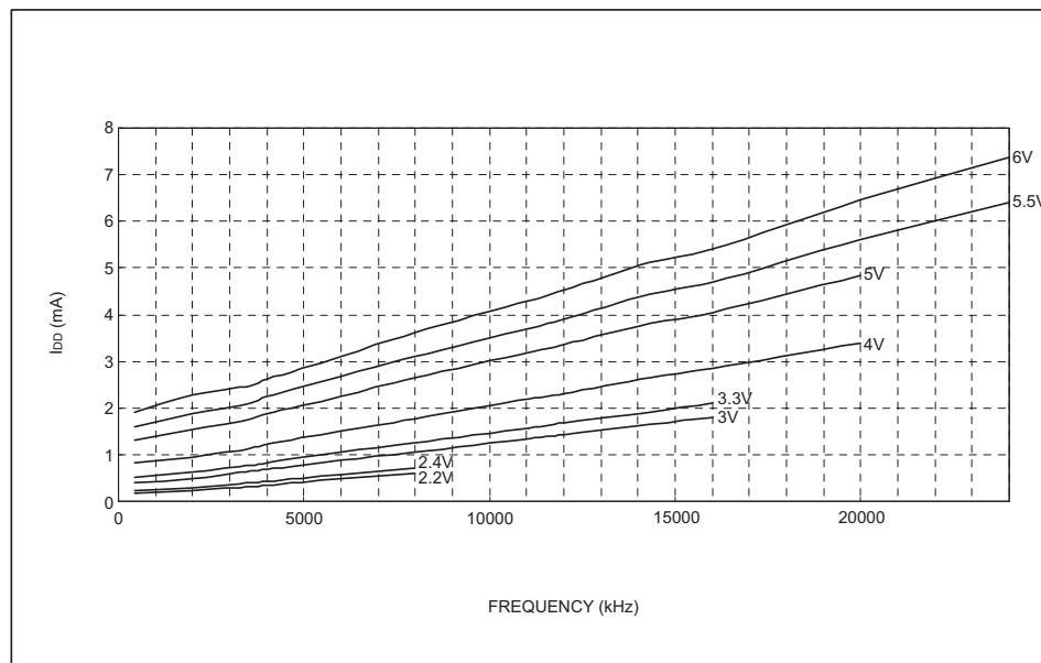
Typical  $I_{DD}$  vs. Frequency (External Clock,  $T_a=0^{\circ}\text{C}$ )
