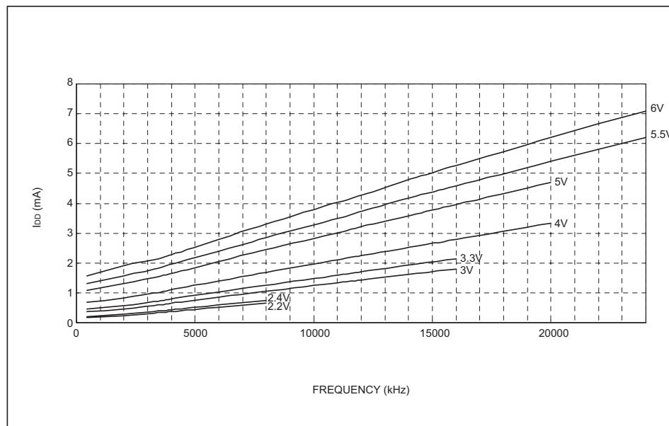
**Typical I<sub>DD</sub> vs. Frequency (External Clock, Ta=+85°C)**
