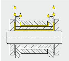
The lubricant product must be able to penetrate into the bearing area of the chain. To guarantee this the lubricant must be applied deliberately to the gap between the inner and outer plates.
