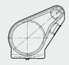
Using enclosed chain boxes and, if necessary, additional centrifugal disc for fastrunning chain drives
