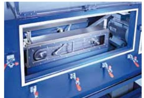
Testing of chain wear elongation behaviour on more than 20 test rigs
