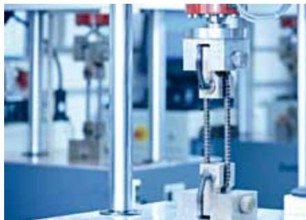
More than 15 pulser are available for testing dynamic fatigue strength according to different testing methods
