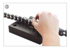
The procedure used is common to both shouldered and parallel bearing pin chains. The new riveting link connects the two inner links. This connecting link is supported by an insert in riveting plate (D) ③.
