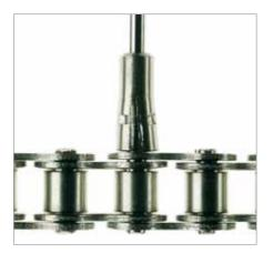
Insert the adapter into the jaws **①** and break it by closing the tool. If necessary, repeat the action after 45° rotation. Once the adapter has been broken, remove the pin.
