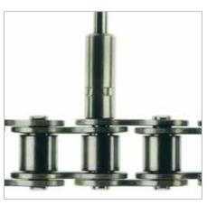
The new adapter is set onto the extended pin. Seize it with the gripping jaws ② and clamp it with the tool. Thus repaired, the chain is operational again.
