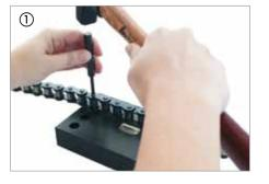
The outer link to be broken has to be placed over the holes in the riveting plate (D). The bearing pins are hammered flush with the outer plate and then driven through the chain with pin punch (B) whose diameter must be smaller than that of the bearing pin **1**.
