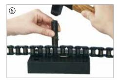
The newly fitted outer link then requires the bearing pin ends to be riveted. This is done with riveting punch (E) **5**.
