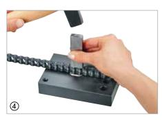
A new outer link plate is fitted using fetching-up punch (C) ④. With parallel bearing pin chain it is possible to over fit the outer link plate on the bearing pins. It is necessary to check that the joint remains free and easily moveble after fitting.
