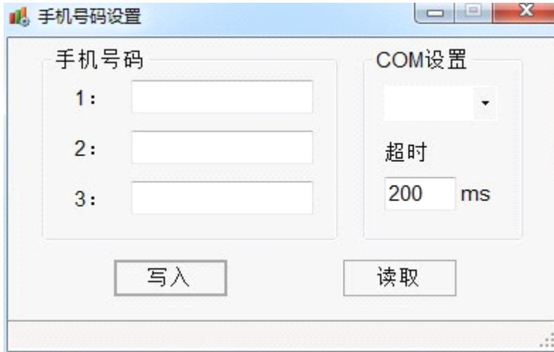
The '手机号码设置' (Mobile Number Setting) dialog box is shown. It contains two main sections: '手机号码' (Mobile Number) and 'COM设置' (COM Setting). The mobile number section has three input fields labeled 1, 2, and 3. The COM setting section includes a dropdown menu and a '超时' (Timeout) field set to 200 ms. At the bottom, there are '写入' (Write) and '读取' (Read) buttons.
