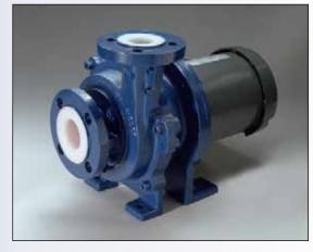
For superior reliability and long life, the ME Series pump utilizes a limited number of wetted components. A standard non-rotating shaft supports a fully encapsulated magnet and fully enclosed impeller. The single rotating bearing is available in a variety of materials for full process compatibility. A PVDF or ETFE rear casing, backed by a fiberglass reinforced plastic shell, supplies high strength containment without sacrificing corrosion resistance.
