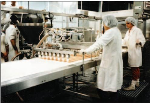
A leading designer and manufacturer of machinery for producing savoury pies, pasties and sausage rolls is incorporating stainless steel W032 pumps into its sausage roll manufacturing machines. Transferring prepared sausage meat in a continuous uniform length to the pastry casing at a capacity of between 5-10m<sup>3</sup>/h, the W range features an auger feeding system to ensure the sausage meat is consistently fed from the extended hopper inlet to the pumping element.
