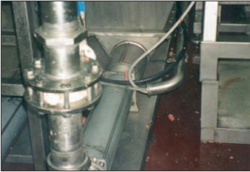
A customer, producing mechanically deboned meats, which are frozen before export to food manufacturers worldwide, has installed a stainless steel W062 pump. The meat puree is gravity fed into the inlet hopper for transfer to the freezer plates. The efficiency of the freezing system relies on a constant flow rate of 5 tonnes per hour, to prevent the plates standing idle or a delay further up the line.
