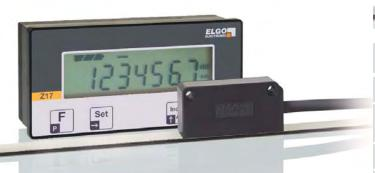
No connections, no effort of wiring, but nevertheless absolute measuring. The absolute position indicators offer more comfort and additional safety. The systems consist of the display unit with a wide range of parameters, and an absolute sensor. This ensures that the actual position is always recorded and displayed. This makes reference runs redundant.
