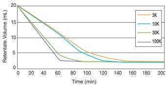
Protein solutions were processed in each of the Macrosep Advance devices. Average time (minutes) is plotted against mL of remaining product to be filtered using a swinging bucket rotor at 5,000 x g. Solutions are 3K: Protamine Sulfate, 0.1% in 1X PBS; 10K: Cytochrome C, 0.025% in 1X PBS; 30K: IgG, 0.1% in 1X PBS; and 100K: Apoferitin, 0.1% in 1X PBS.
