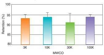
Protein solutions were processed in each of the Microsep Advance devices. Average percent retention using 34° fixed angle rotor at 5,000 g is displayed for each MWCO. Solutions were 3K: Cytochrome C, 250 µg/mL; 10K: BSA, 1 mg/mL; 30K: lgG, 1 mg/mL; and 100K: thyroglobulin, 1 mg/mL.
