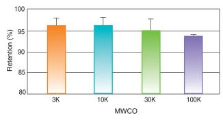
Protein solutions were processed in each of the Macrosep Advance devices. Average percent retention using a swinging bucket rotor at 5,000 x g is displayed for each MWCO. Solutions were 3K: Protamine Sulfate, 0.1% 1X PBS; 10K: Cytochrome C, 0.025% in 1X PBS; 30K: IgG, 0.1% in 1X PBS; and 100K: Apoferritin, 0.1% in 1X PBS.
