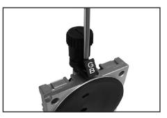
Loosen connection fastener slightly.
