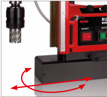
Standard fine adjustment stabilised • Displaceability: \pm 10 mm • Pivoting range: \pm 30^\circ
