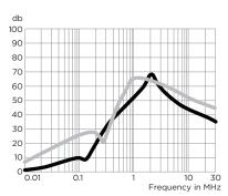
Minimum Insertion Loss - Measured in closed 50 Ohm system
