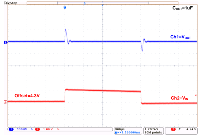
Line Transient at V_{OUT}=3.3V : ( I_{OUT}=10mA )
