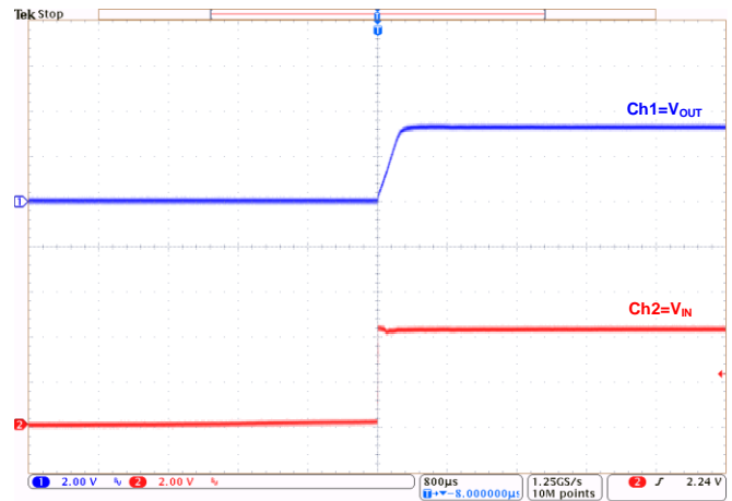
Power-Up at V_{OUT}=3.3V : ( I_{OUT}=500mA )
