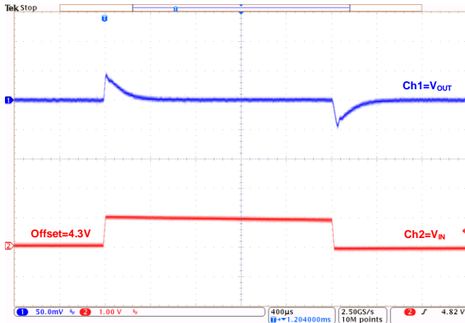
Line Transient at V_{OUT}=3.3V : ( I_{OUT}=1mA )
