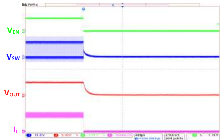
Figure 16. Shutdown Through EN, I_{OUT}=0.6A
